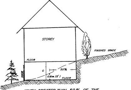
WHEN GREATER THAN 50% OF THE FLOOR AREA IS NOT LESS THAN 0.61 m (2') BELOW GRADE, AND WHEN THERE IS AN ENTRANCE/EXIT AT GRADE LEVEL THEN 'C' IS A WALKOUT BASEMENT
